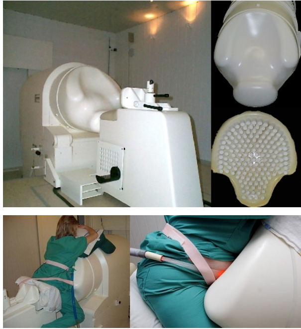
Figure 1: Multi-channel superconducting quantum interference device (SQUID) system.
