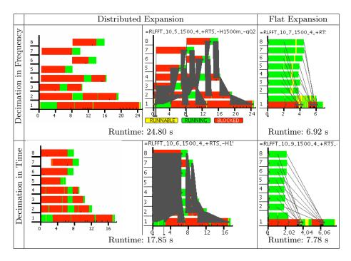
Fig. 3. Traces and runtimes of divide-and-conquer approaches, without/with messages.
