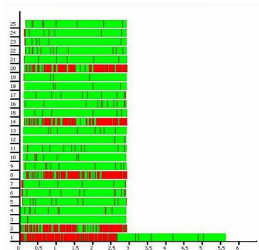
Fig. 34. Mandelbrot trace on 25 PEs with hierarchical master-worker skeleton (hierarchy shown on the right)
