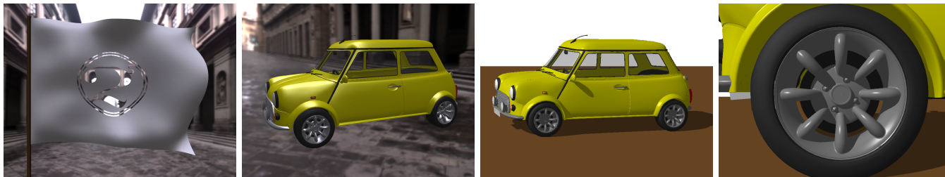
Figure 1: Rendering of NURBS models (from left to right): animated trimmed NURBS surface (degree 5 \times 5 , 100 control points) with environment mapping; Mini model consisting of 629 trimmed surfaces; with shadow maps; closeup onto the front wheel.
