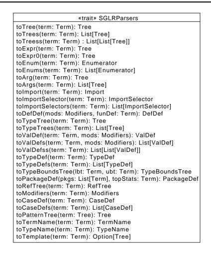
Figure 4.2.: List of methods used for the transformation of Term to Tree
