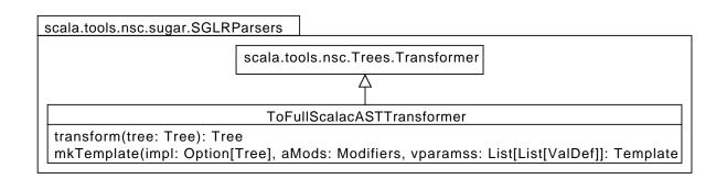
Figure 4.4.: Signature of the transformer from intermediate *Tree* nodes to the native Scala AST
