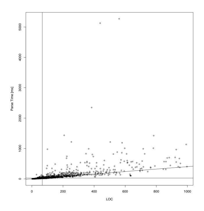
Figure 2.4.: Parse times for the 1482 successfully parsed files with LOC  $\leq$  1000 – lines mark medians and resulting gradient through origin
