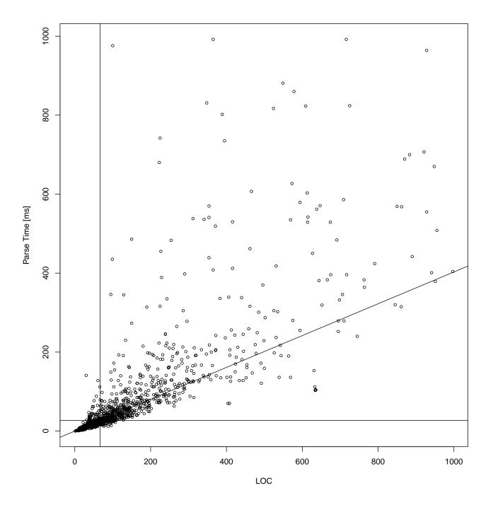
Figure B.1.: Parse times for the 1471 successfully parsed files with LOC  $\leq$  1000 and parse time  $\leq$  1s – lines mark medians and resulting gradient through origin
