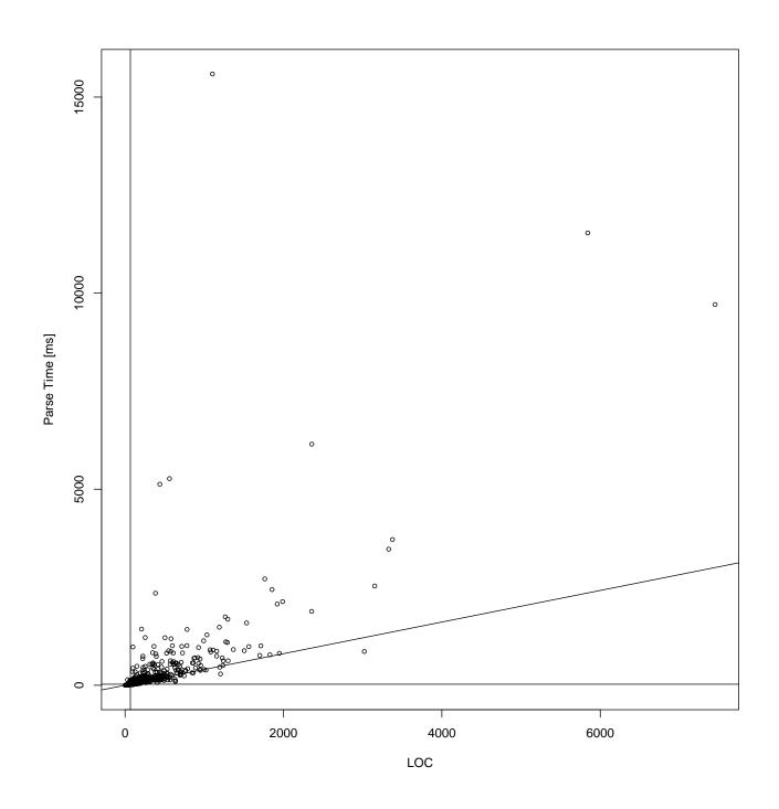
Figure 2.3.: Parse times for all 1521 successfully parsed files — lines mark medians and resulting gradient through origin
