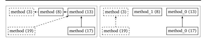
**Figure 3.2:** Name graphs for the example program from Fig. 3.1 (left) and the version insufficiently renamed by NameFix (right). Synthesized nodes/edges are dotted, class names are not included for clarity reasons.
