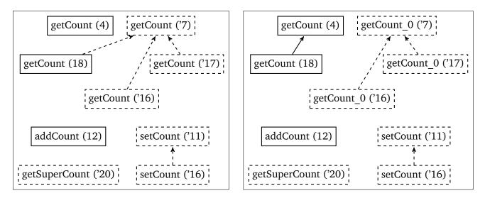
Figure 2.7: Name graphs for the transformed example program from Fig. 2.3 (left) and the result after NameFix is applied. Class/field names are not included for clarity reasons.
