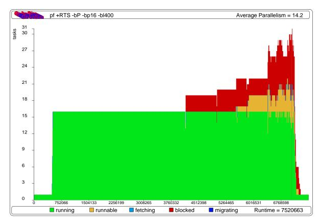
Overall, for this simple program the utilisation is almost perfect as the green (medium-gray) area reaches up to 16 almost through the whole computation. Only at the end of the computation there is a significant number of runnable (amber or light-gray) and blocked (red or black) threads.
