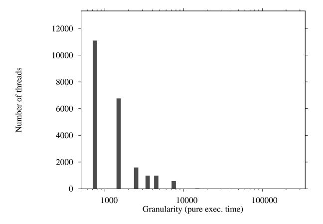
It shows that this program creates a huge number of tiny threads (note the log scale in the graph). Refining the intervals for these tiny threads further gives the following bucket statistics
