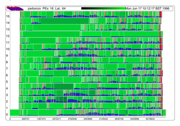
The graph shows the activity of each of the 16 processors in this simulation. The dark green areas in the first third of the computation show that processors 2, 4 and 14 have a significantly higher load of runnable threads than the rest. Also note the pattern that a decreasing number of blocked threads (thinner blue bar) is accompanied by an increasing number of runnable threads (darker green area).
