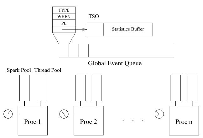
GranSim performs an event driven simulation with a centralised event queue. Each of the simulated processors has its own spark queue and thread queue as well as its own clock. The
