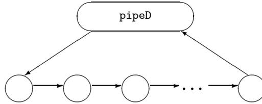
Fig. 9. Intended pipeline topology
