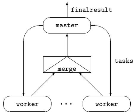
Fig. 10. Master-worker process topology
