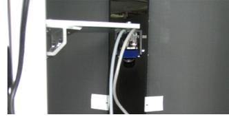
Figure 3: Camera mounted between two projection screens. Note that while the view direction can be modified, the up vector of the camera is fixed.
