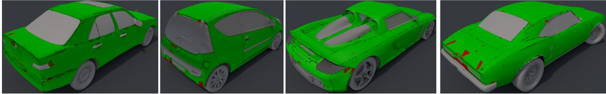
Figure 8: Visualization of the coverage for three of the models used during the optimization. Green is covered, red is not covered, black is not externally visible. The rightmost image shows the coverage of a car that was not part of this set. Nevertheless, we still achieve a good coverage.
